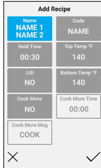
Key information on each recipe is displayed on this screen view. This includes the Recipe Name (appears on the well on the runtime screen), the Hold Time, Cook More Time, Top Temperature and the Bottom Temperature.
